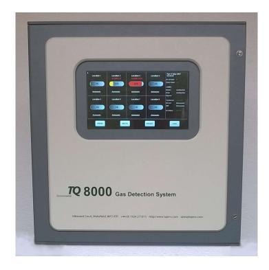
The New **TQ8000 Touch** is an 8 channel stand-alone control unit, which can be expanded up to 48 channels for larger installations. Capable of monitoring inputs from a wide variety of TQ Environmental Gas Detectors and many other 4-20mA output devices, such as temperature, pressure and PH sensors
